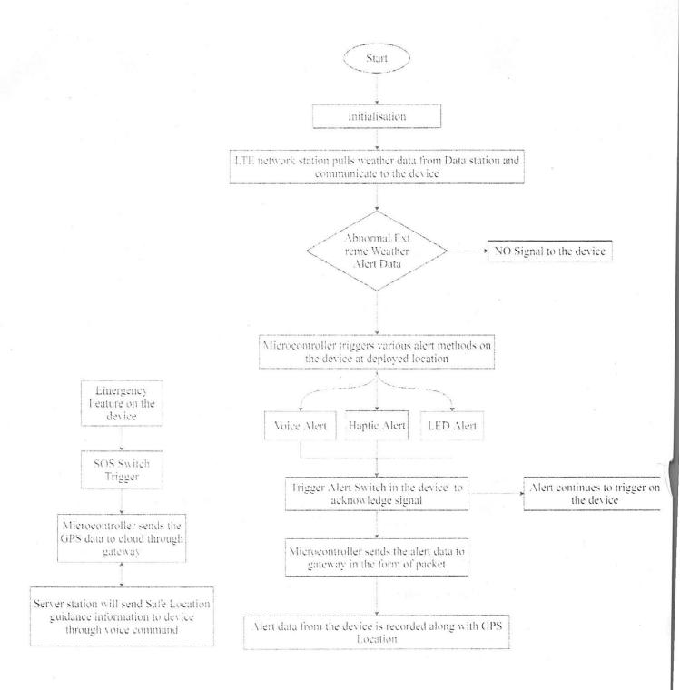
Flowchart of operating process of the weather alert system
